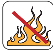
Flame Retardancy NF C32-070-2.1(C2) IEC60332-1-2/EN50265-2-1
